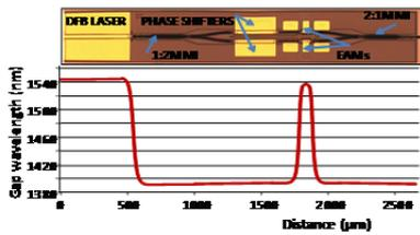
Fig 1. SAG PL design for each photonic function of a BPSK PIC
