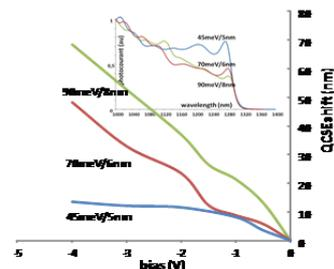
Fig 3. Measured QCSE shift and absorption spectra for 3 QW designs
