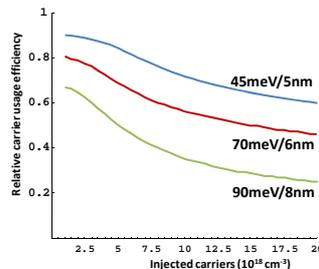
Fig 2. Simulated internal efficiency for three QW designs
