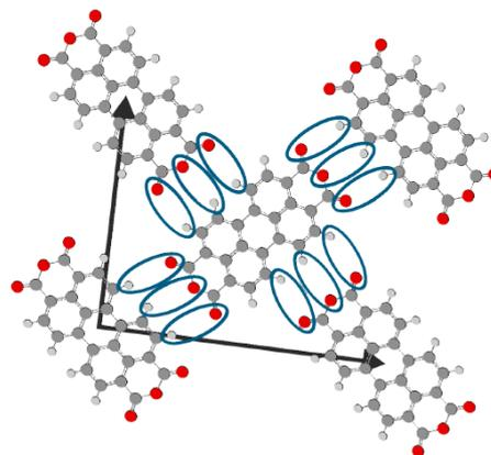
Figure 2: Molecular arrangement of PTCDA on Cu(001). Hydrogen bonds are indicated as blue ellipses.
