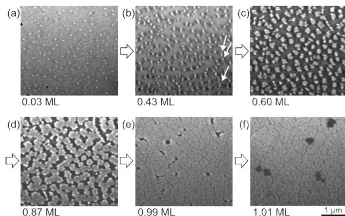
Figure 1: LEEM images obtained during the growth of PTCDA on Cu(001) at 350K. PTCDA islands appear bright, clean Cu(001) areas dark. Start energies of 2 V (a, b) and 1.3 V (c-f) and slight under-focus conditions were used.
