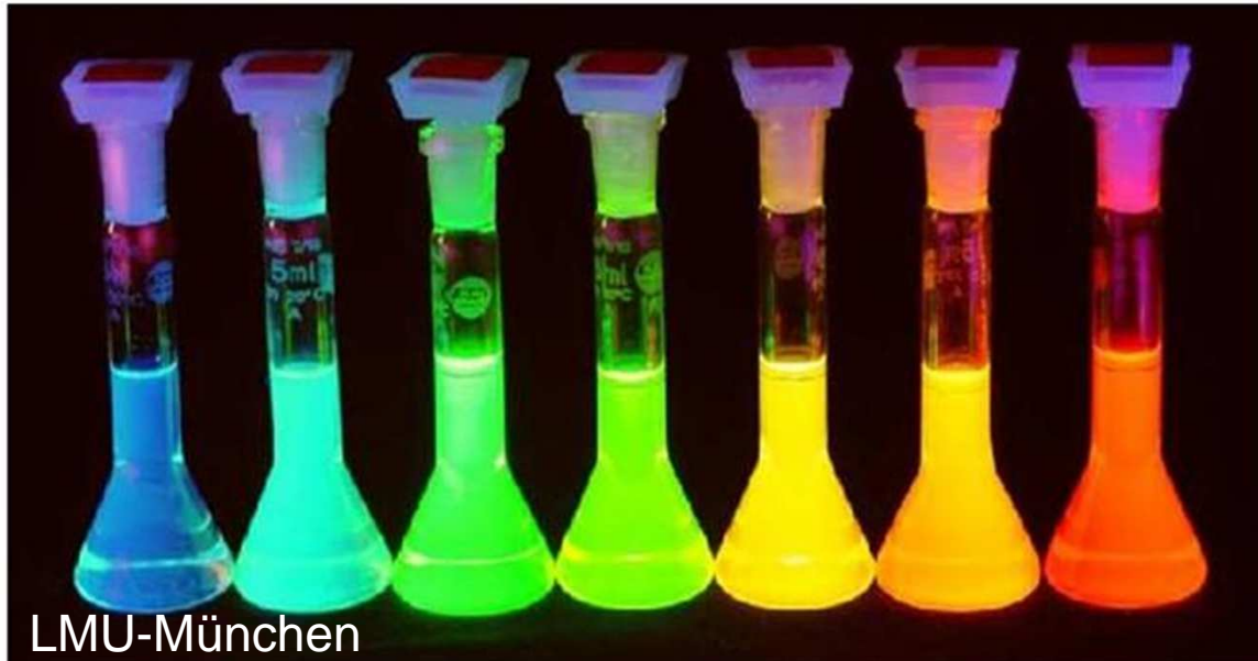
Fluorescence image of CdSe QDs in solution with size 2-6 nm
